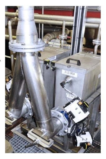
The Separation quality can be adjusted by selection of the utilized separator blade hole size, with **finenesses ranging** from **1.000 to 10.000 µm** available.
