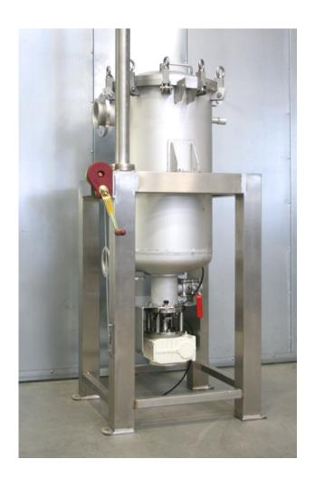
In our design, the filter basket is continuously cleaned by **spring loaded doctor blades** (scraper). This ensures a fully automatic filtration process that maintains very low pressure differences, **typically below 1.0 bar.**
