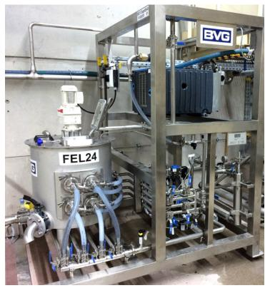
The deaeration process takes placeinside an agitated tank where the optimum distribution of product on the membrane surface can be controlled.
