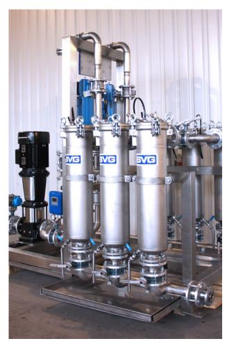
The *Strainer B* is a simple, and operator friendly system. Increase of differential pressure determines the required change of the filter bag. A mechanical hoist is used by the operator to remove the used filter bag. Suitable for the **filtration of Newtonian fluids**, a typical application is in **chemical dosing** lines for solutions. The filtration degree can be adjusted by selection of the utilized filter bag, where different materials and finenesses between 1 to 500 µm are available.
