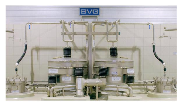
The **Separator V** is a **vibrating screen** for applications in the pulp & paper industry (and others) where coarse particles have to be removed while they are considered as out of specification while specific smaller particles must be retained. Typical applications are grinding or dispersing system for pigments and minerals.
