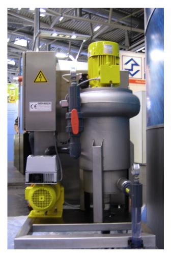
This scraper design optimizes the filtration efficiency and flow circulation of the *Cyclone Filter W*. The separation quality can be adjusted by selection of the utilized filter element, where different **finenesses** between **25 to 1.000 \mu m** are available.
