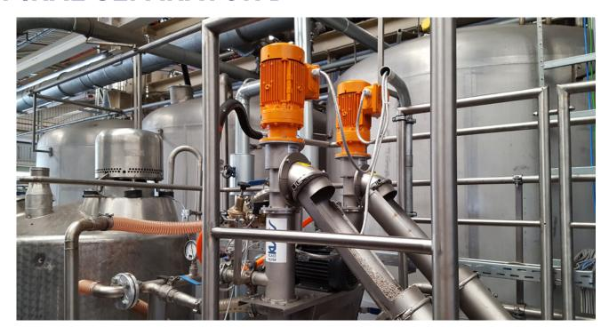
The *Spiral Separator D* is a system for solid-liquid separation applications in the pulp & paper industry (and others) where a separation into a dry substance is required (stock preparation, flotation foam, wastewater treatment). By using a turning spiral inside a filter element, the solid particles are transported continuously and simultaneous dewatered with the aid of a drain pump.
