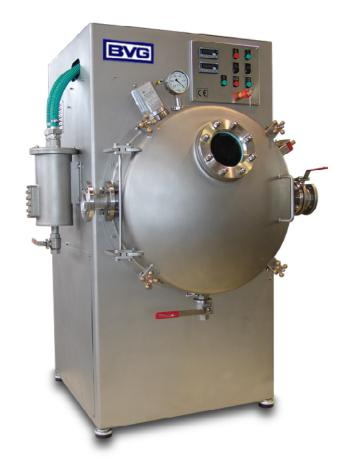
By centrifugal force a thin product layer is formed on the rotating roll and is constantly deaerated. After the deaerated product is deposited on the edge of the rotating bowl, a pick-up pipe discharges the product out of the *Super ExAir TL*. Due to its compact design, the *Super ExAir TL* can be installed on the same level as the working station (no vertical height required).
