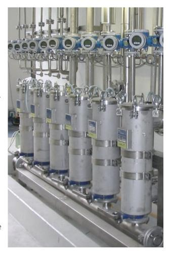
The Strainer C is ideal for **filtration of non-Newtonian** (solids containing) **fluids** such a pigment slurries, dispersions, starch glue, and coating color. A typical set-up is the function of a **police filter** in product dosing lines.
